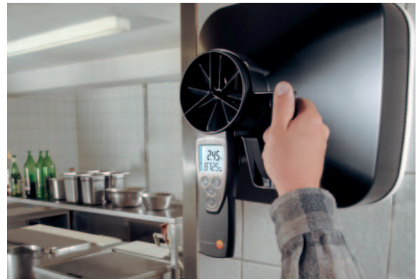
testo 417 monitoring the exhaust air flow at a wall duct
